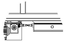
Figure 35: Connection between trolley and end carriage **STEP 6:** in this step, installer must begin the installation of the power driven trolley inside cross bridge. First, one track end stop must be removed. Then the cross bridge trolley can be removed.
