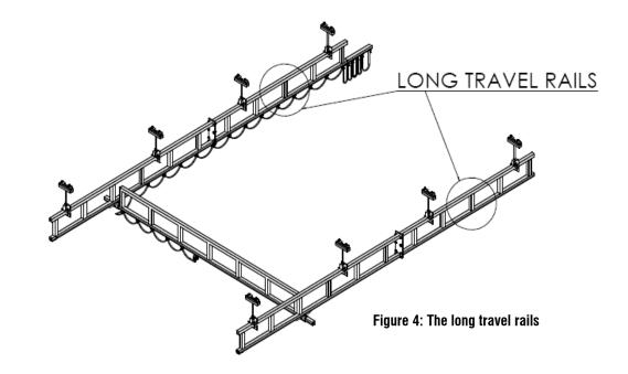
This is the first stage of the installation procedure. Long travel tracks are installed using the supports suggested by the manufacturer. This stage includes three separate steps:
