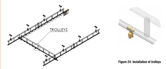
With one side open (as described in previous paragraph), load bearing trolleys can be inserted into the cross bridge. There are many different trolleys. Some of them are as follows:
