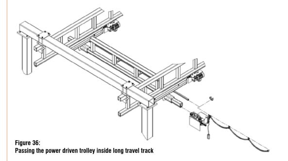
**STEP 8:** the trolleys have to be reinstalled inside the cross bridge. Please note: trolleys and power driven trolleys have to be oriented in such way that connection will be possible.
