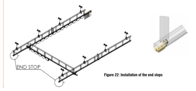
Once both long travel tracks and cross bridge have been installed, track end stops must be placed at all track ends. This is crucial for safety reasons in order to avoid any fall from height, with the exception of one side of long travel track which has to remain open in order that cable trolleys can be fed into the rail. Also, one side of cross bridge has to remain open because the trolley has to be inserted.
