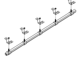
**STEP 3B:** in this case two halves of the support must be bolted together on either ends of the track. With this, the long travel track can be positions between the two support halves and secured by tightening the cross bolts to the steel structure. Then, all the other supports can be installed consecutively in the proper positions.
