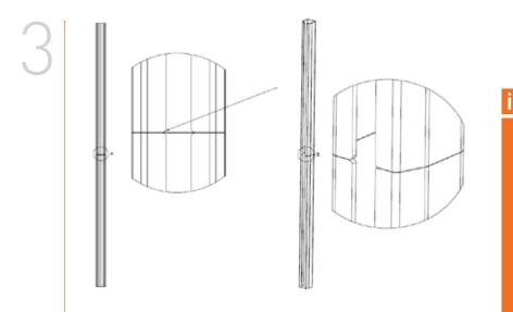
Figure 7: The right preparation of two parts of track in order to get joined
