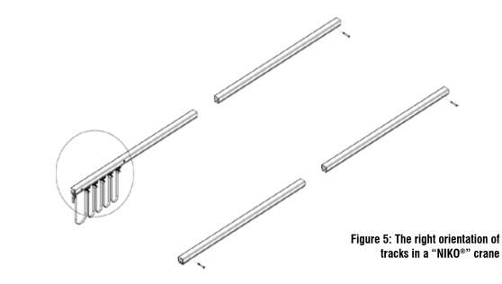
✓ If there is track with two holes, it will be used at the extremities of the long travel rails inside which both end carriages and cable trolleys will move. The side with two holes will be used for parking cable trolleys. One of the two holes will be used for type .X06 transverse bolt which stops end carriage movement. Cable trolleys can pass under this bolt and bunch up within the parking area. The other hole is used for the extra transverse bolt which accompanies end stop .X01.
