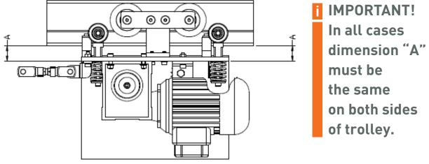
Figure 40: Dimension "A" for power driven trolley
