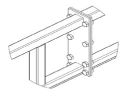
In this case, all the bolts are bolted progressively so that the best alignment is achieved. This must be checked during the maintenance process.
