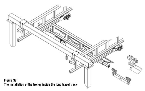
**STEP 9:** in this step the power driven trolley will connect to the trolley.
