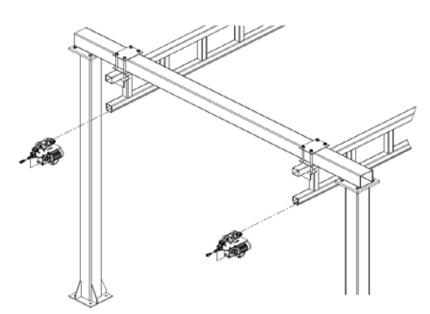
**STEP 4:** the set of cross bridge and end carriages can now be re-installed. Installer has to take into account the orientation of the set. It has to be in such way that connection with power driven trolleys is possible (see figure below).
