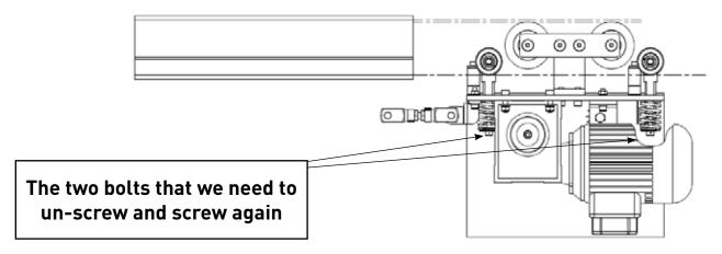
Figure 39: Adjustment screws for power driven trolleys
