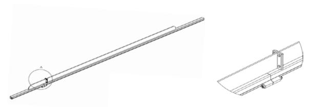
Figure 14: Junction using special plate and chocks
