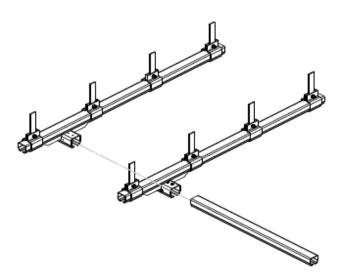
Figure 20: Installation of the cross bridge using the free side of the construction
