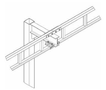
Figure 16: Junction using ".Z13" type support
