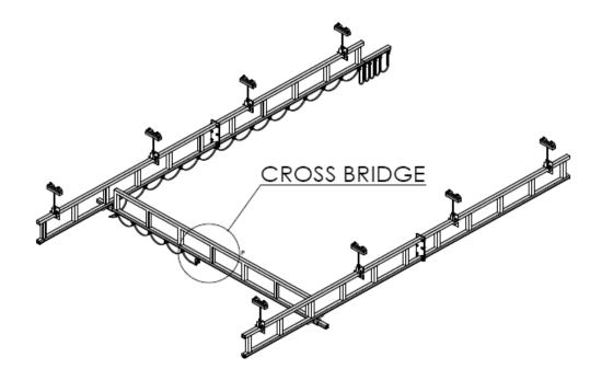
Figure 18: The cross bridge in a "NIKO®" crane
