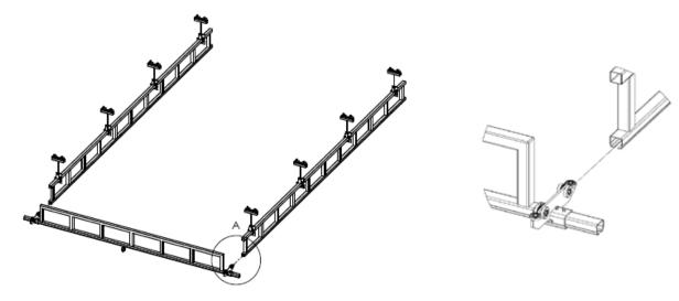
Figure 21: Installation of a cross bridge with reinforcement
