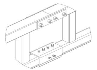
It is a very common way of junction due to easy installation. The splice joint must be installed as it is described in paragraph 3.2.2.1. Extra flanges are used to join the two parts of the square profiles and to align each other. This is will be achieved tightening progressively the bolts of the flanges.
